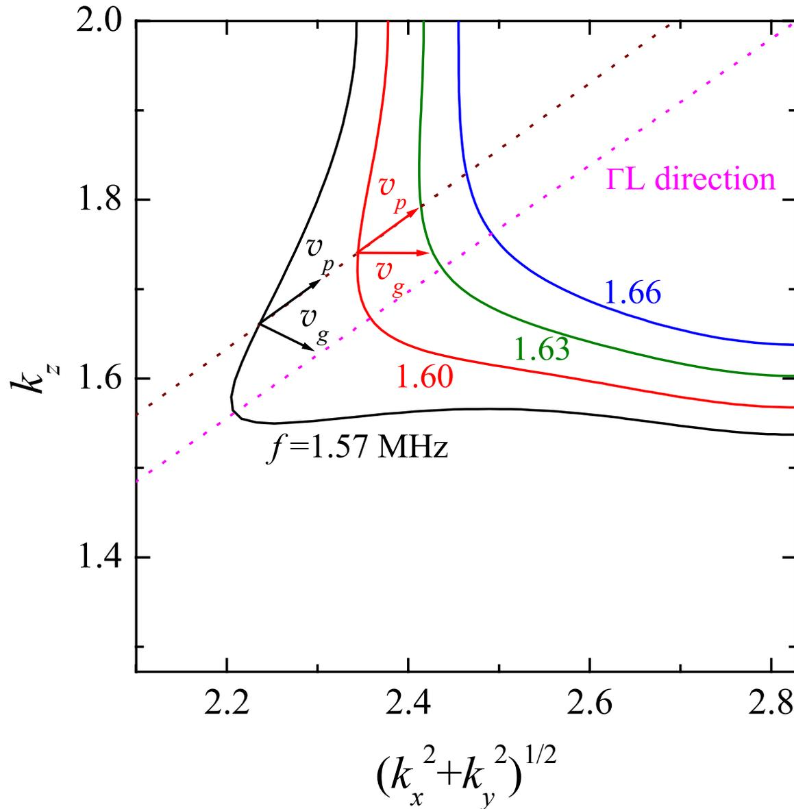
The direction normal to the dispersion surface is the wave transport direction, since
